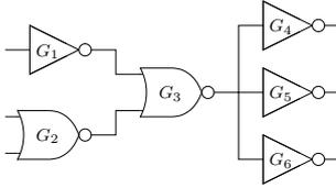
Fig. 2: Fan-in and fan-out correlation example circuit.
