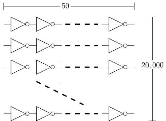
Fig. 6: 1M inverter test circuit.
