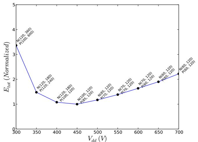
Fig. 7: Results of the reliable-circuit minimum energy algorithm applied to 1M inverter test circuit with  $P(L,W)$  and  $N(L,W)$  given for each point in nanometers.
